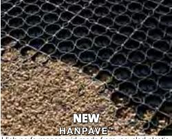
High performance grid made from recycled plastic. Designed for car-parking. Can be filled with earth or gravel. Allows rainwater to pass at a controlled rate. SuDS compliant.
