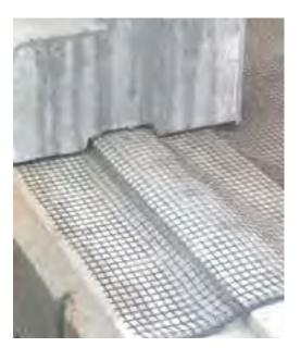
A geogrid is a mesh-like system integrated into the construction of driveways and retaining walls to reinforce soil & gravel by providing additional support and redistributing the weight of pressure placed on the surface, across a wider area. Geogrids are manufactured using polymers (polyester, polyethylene) known for their tensile strength and durability.
