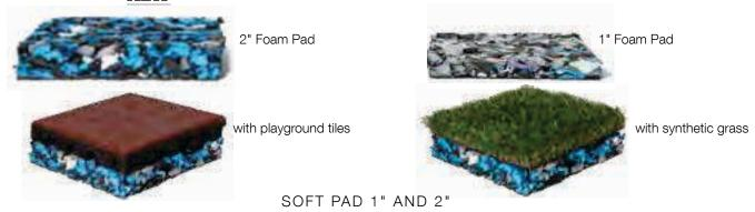
Creates safety impact for play areas and playgrounds. IPEMA approved and developed to allow water to drain through to the sub base, reducing the need for aggregate and expensive drainage systems. Can be customized for fall heights up to 12'. 4' x 6' sheets.
