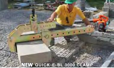
The ultimate tool for picking step treads, slabs and wall material. Can pick product from front-to-back, or up to 4' end-to-end. Clamp adjusts from 9" - 48" and holds up to 1800 lbs.
