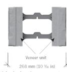
double sided plastic connector tandem wall: 2D view
