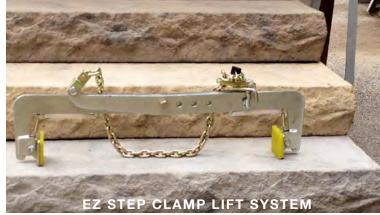
Comes in 3 sizes with an optional hook attachment for use with installation equipment. Perfect for lifting various materials including natural stone steps, curbing, & large stone retaining walls. Available in: 900 lb. capacity (max. width 28"); 2400 lb. capacity (max. width 42"); 3000 lb. capacity (max. width 50").
